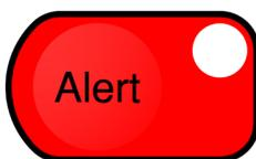
In MANUAL when **Alert** is pressed the alert signal will be generated in the particular zone. Pressing the key again will turn off the alert signal. Note that if **Evac** was active for the zone pressing **Alert** will clear the Evac signal.
