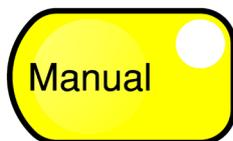
If **Manual** is pressed MANUAL is requested for the ECP. If MANUAL is granted the associated **Manual** LED will turn on steady and **Auto** will be turned off. If only some zones are placed in MANUAL then the LED will flash (the AUTO LED will also remain on).
