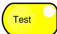
If **Test** is pressed the QE20 enters Test Mode and any warning signals activated will not be generated in their zones, but just indicated on the ECP. The associated **Test** indicator will turn on to show that TEST is active. Refer to Section 3.5 for more details about TEST. The QE20 must have no zones in Alert, Evac or Speech and Silence Warning must be off to enter Test Mode.
