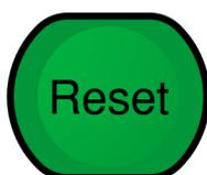
If **Reset** is pressed in MANUAL and when **Silence Warning** is on, all latched alarm and fault indications will be reset and cleared, plus all Zones in the Alert, Evacuate or Speech will be cleared. Any alarm or fault conditions that are still physically present (e.g., fire panel alarm or MCP activated) will remain. These will need to be cleared at their source and then **Reset** before pressing **Auto**.
