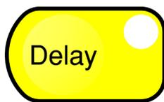
If **Delay** is pressed Delayed Alarm Operation will be selected, if configured (note it may be a delay of 0 seconds). The **Delay** LED will turn on.
