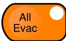
When **All Evac** is pressed all zones are placed in the evacuate state and the **All Evac** LED is turned on. Each zone **Evacuate** LED will also turn on to indicate it is in evacuate.
