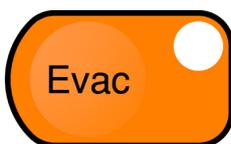
In MANUAL when **Evac** is pressed the evacuate signal will be generated in the particular zone. Pressing the **Evac** key again will turn off the evacuate signal. Note that if Alert was active for the zone pressing **Evac** will clear the Alert state.
