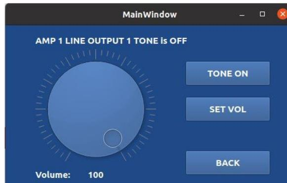
On this screen the volume for the amplifier can be adjusted from 0 to 100% by rotating the rotary control to the required setting and pressing the **SET VOL** button. This will change the volume for that amplifier for all audio functions and the setting will be saved in non-volatile memory so it is not lost.
