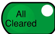
When **All Cleared** is pressed the **All Cleared** LED and the **Zone Cleared** LED for all configured zones will be turned on. If the **All Cleared** LED is already on pressing **All Cleared** will turn this LED and all configured zone **Cleared** LEDs off. This is basically a log indicator and has no effect on system operation. It provides helpful information to the operator. It could be used to indicate each floor has been evacuated.
