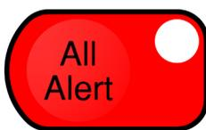
When **All Alert** is pressed all configured zones are placed in the alert state and the **All Alert** LED is turned on. Each zone **Alert** LED will turn on to indicate it is in alert.
