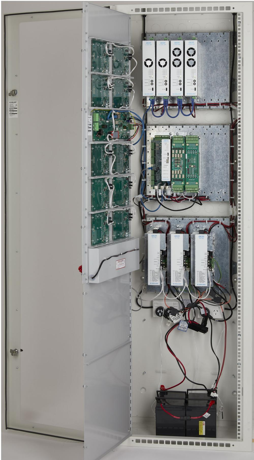
Figure 3 Example QE20 Internal View
