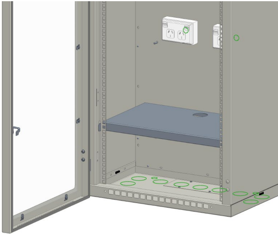
Figure 4 –Lower Battery Shelf into place in QE20 Cabinet
