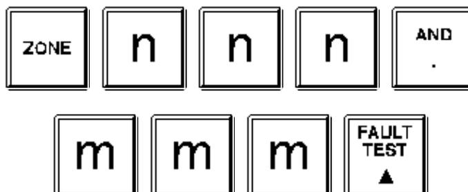
The LCD will display the range of zones selected. Press the "ACK" key to initiate the alarm test or fault test of zones nnn to mmm inclusive or press the "CLEAR ESC" key to abort. The RDU will not initiate a test on any zones within the range that do not have this command enabled.
