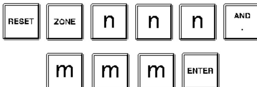
The LCD will display the range of zones selected. Press the "ACK" key to initiate the reset of zones nnn to mmm inclusive or press the "CLEAR ESC" key to abort with no reset.
