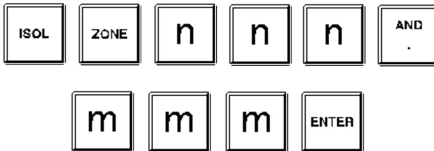
The LCD will display the selected range of zones, i.e., zone nnn to zone mmm inclusive, plus the options to isolate or de-isolate the range.
