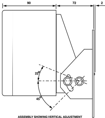
Fig. 3 Clearance Required for Full Adjustment
