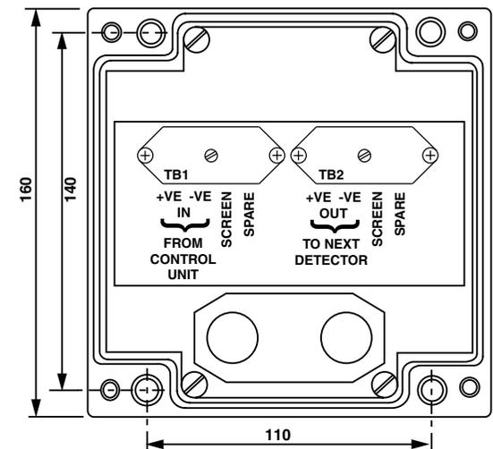
Fig. 2 Fixing Dimensions
