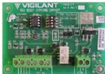
The ISO 8201 Strobe Driver generates an ISO 8201 compliant "T3" pattern for the Multi-Candela strobe 4906-9104.
