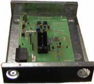
The IO-NET Programming Unit transfers the program to the IO-NET Controller PROMs. The Programming Unit is supplied complete with a cable to connect to a PC, the compiler programming software and the user manual. An external 24Vdc supply is required. IO-NET is also able to be programmed using SmartConfig Version 1.6 onwards. If the IO-NET site specific configuration is stored in read-only memory. It may be re-programmed multiple times before requiring replacement (SF0239).
