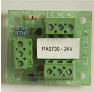
The 24V PA0730 two pole changeover contact general purpose relay board may be used in either of two modes:
