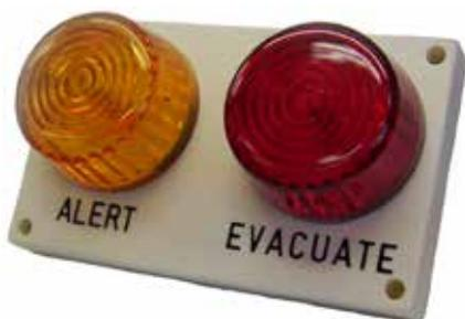
Where two distinct visible signals are required, the VIGILANT EA0313 Dual Strobe unit is available. The dual strobes operate at 24 volts and provide a 2.6 Joule output. The strobes may be powered in tandem over a two wire circuit or independently over a 4 wire circuit.
