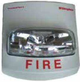
The 4906-910x Multi-Candela strobe is a high output xenon strobe capable of signalling evacuation using the ISO 8201 "T3" temporal pattern, as required by AS1670.4-2004 and AS 1670.1-2004. It produces white light with a link-selectable intensity of 15cd, 30cd, 75cd or 110cd. It is controlled by either the ISO 8201 Strobe Driver Module (PA1043) or a QE90 STRM Strobe Relay Module (PA0697).
