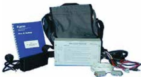
Provides alarm test for detectors that support it. The MX Loop Tester allows Walk Test. Any device going into alarm is shown on the laptop with address and time. Walk Test Status (devices not tested yet) can be requested. Walk test mode overrides detection algorithm delays for fast testing.
