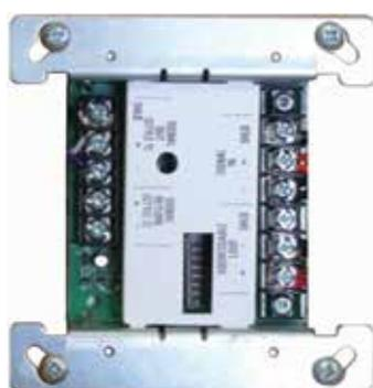
This IDNet addressable device provides a supervised, addressable interface to conventional warning devices such as sounders or strobes. The Signal IAM requires a supervised power supply or compatible signal input for powering the externally connected loads.
