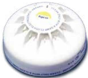
The MDU601EX detector combines the features of both the MU601EX detector and the MD601EX detector to provide a combined CO and Rate of Rise Heat Detector where the sensitivity of the CO detector is enhanced in response to a fast rate of change of temperature.
