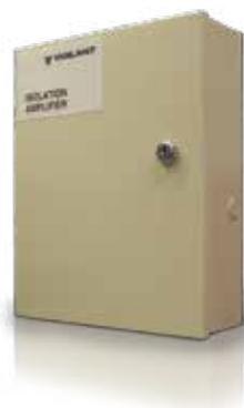
The FP1135 T-Gen2 Isolation Amplifier connects to an existing 100V speaker line and reproduces this signal at up to 60W load on a separate supervised 100V line. It is suitable for use with speech and music as well as with warning tones. The 100V output line from the amplifier is electrically isolated from the input 100V line, so noise or other signals on the output line are kept separate and do not affect the input line.
