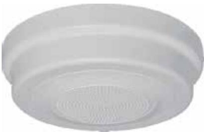
EA0031/33 are designed to mount directly to the underside of concrete slabs or inaccessible ceilings. The housing is surface mounted with concealed internal fixings. Speaker cable entry can be either from the rear, or via surface mounted conduit (four 19mm conduit knockouts are provided).
