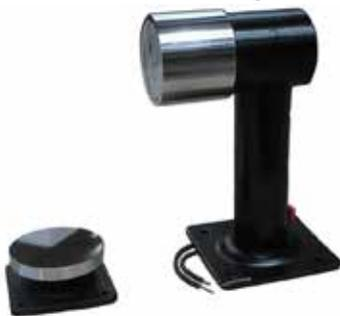
The EA0410 Electromagnetic Door Holder is designed to hold fire and smoke doors open under normal conditions, but automatically close under their own spring return mechanism when a fire or smoke alarm system is activated. The door is held open by the magnetic force between an electromagnet mounted on the wall behind the door and a keeper fixed to the back of the door. When the electrical supply to the electromagnet is de-energised and the door automatically closes.
