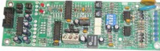
**PA0773** RS485 Comms CMOS PCB 1901-139-3 FRC only (FRC connection - including power). The PA0773 is used to interface an F3200 FIP, MX4428 FIP, PTM, NLDU, MODBUS BRIDGE, RDU or NDU with the RS485 network. This RS485 Communication Board is mounted on four metal stand-offs, which are used for earthing the PCB. This RS485 board connects to the controller board via a 10 way FRC LM0172 (ordered separately), which is also used to power the RS485 Board.
