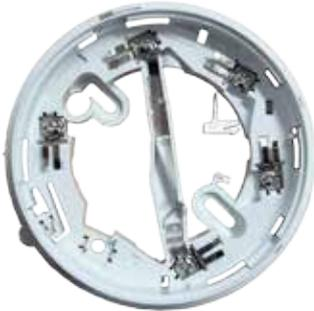
The 4B-C Continuity Base is used for most installations involving 850 Series detectors, as it allows the detector's in-built short circuit isolation function to be in-circuit when the detector is fitted and ensures continuity is maintained when the detector is removed.
