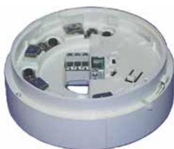
The 814RB Addressable Relay Base provides two sets of changeover volt-free relay contacts capable of switching 1A (resistive) @30Vdc. The relay function is controlled by the MX fire alarm panel via the detector fitted to the 814RB. The 814RB may be mounted to the ceiling, plugged into an M614/5B Universal Base or an 5Bl/814IB Isolator Base. **Use with MX1, MX4428.**
