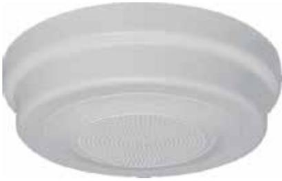
EA0029 is designed to mount directly to the underside of concrete slabs or inaccessible ceilings. The housing is surface mounted with concealed internal fixings. Speaker cable entry can be either from the rear, or via surface mounted conduit (four 19mm conduit knockouts are provided).
