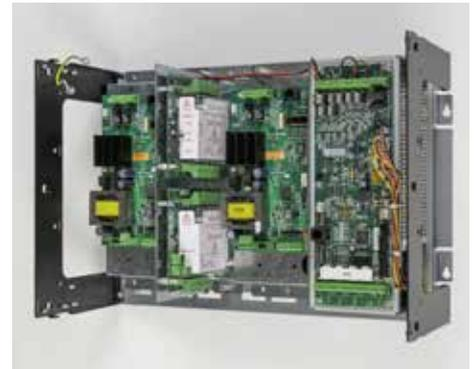
**T-GEN 60** on FP1119 Bracket in PDI Expansion Bay with FP1118 Brackets & Splitter Modules
