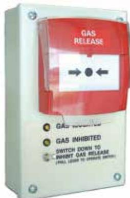
**FP0570** Local Gas Control Station - Automatic. Local Gas Control Stations (LGCS) are used in gaseous fire extinguishing systems to provide local area manual control of a release. The automatic version includes a Gas Inhibit switch, buzzer and LED, whereas the manual version (FP0572) does not. The LGCS is fitted with a resettable no-break plastic frangible element.
