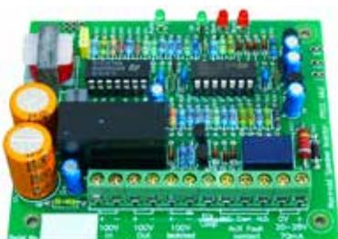
To prevent PA loudspeakers in a secure area from being used as microphones, the Speaker Isolation Module SIM-Mk2 is installed within the secure area between an incoming 100V speaker circuit and the speakers to be secured.
