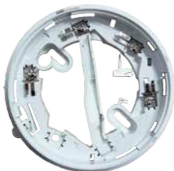
The 4B Universal Base contains no electronics and is suitable for indoor applications of the 614 series conventional (non-addressable), 814 and 850 series analogue addressable detectors. It provides excellent space for cable access and terminations. It features remote LED connections and an anti-tamper facility. The 4B base is designed to snap-fit into the ceiling tile adaptor, or screw fix to the ceiling in the traditional manner.
