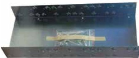
A KT0072 Cardframe upgrade kit can be fitted to a 15U F3200 to allow it to take more than three 8 way modules. The KT0072 cardframe can accommodate 8 F3200 modules (for MX4428:- 8 ADR or 6 MPR/MXP/ADR+RRM). In older versions, the cardframe mounts directly to the rear of the cabinet. In newer versions, the cardframe is fitted to a gear plate that may be removed when the cabinet is mounted to the wall.
