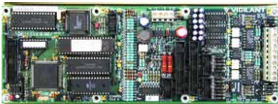
The Panel-Link Modbus Bridge (PMB) is designed to translate data from VIGILANT fire alarm systems on a Panel-Link network to a Modbus communication line. The PMB not only monitors the Panel-Link network, but also provides a means of direct control over the fire systems. The PMB database contains data on the states
