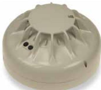
The 850H is a flexible cost-effective addressable heat detector with most of the features of MX VIRTUAL detectors. The 850H reports the temperature to the MX fire alarm panel which allows various detection modes. The 850H uses a high quality thermistor with very low thermal mass. This allows the detector to function as a heat detector as well as providing a fast and accurate temperature display. **Use with MX1, MX4428, 4100ESi.**
