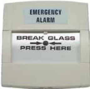
The SU0608 MCP is surface mounting, with a plastic coated glass element to ensure reliable, safe operation. It is coloured white (for EWIS applications) to be used where a fire alarm system does not exist. The call point is operated when the glass element is snapped, releasing the MCP's micro switch, which signals an alarm to the EWIS panel. The element is snapped by pressing on its centre – a hammer, or other impact device, is not required.
