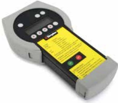
The Simplex TrueSTART II Test Tool is a portable battery-operated test instrument, designed to enable contractors or technicians to quickly verify that all IDNet wiring and peripheral devices are installed correctly and operating properly, even before they are connected to the 4100 fire alarm control panel.
