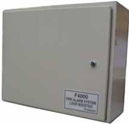
The MX4428/F4000 Loop Booster overcomes problems such as Responder loop voltage drop and excessive loop length that would otherwise necessitate a restriction in responders or the use of thicker loop cable. By providing additional power supply capacity to an MX4428/F4000 loop, the Loop Booster is a practical and cost-effective means of overcoming these problems, thus enabling extension of the loop length, additional
