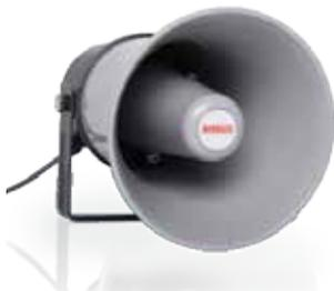
The EA0020 is a high performance 8 ohm horn speaker for use in smaller PA applications requiring a low impedance audio solution. It is ideal for use as an external sounder for the VIGILANT IP65 AVI Mk2 where increased warning tone volume is required. The EA0020 should be mounted adjacent to the IP65 AVI Mk2. The cable supplied with the speaker should enter the AVI using the supplied 16mm cable glands and be terminated at the AVI Controller board.
