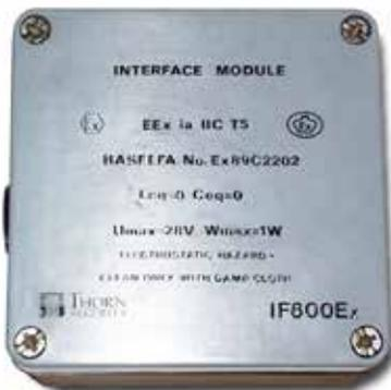
The Intrinsically Safe IF800Ex Interface Module is designed to monitor fire contacts such as extinguishing system controls, ventilation controls, fire door controls etc. The IF800Ex is contained within a grey compression moulded glass filled polyester box with 3 x 20mm cable gland holes. The electronic components are mounted on a double sided printed circuit board built into a potted module formed from a plastic moulding. Connectivity is via two terminal blocks fitted to the circuit board.
