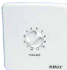
These 100V line audio attenuators install in a standard electrical flush box or mounting block. Screwdriver terminals enable a simple and neat connection. Models for 10W, 40W and 100W have an override relay facility. With fire evacuation systems it is necessary to override the attenuator setting to broadcast an announcement at full volume. The override relay requires 24Vdc to allow the attenuator to operate normally. This 24Vdc can be provided from the QE90 Amplifier Transformer Relay Output.
