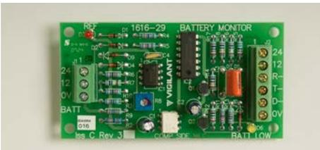
The Battery Monitor is a small module designed to provide supervision of supplementary 12 or 24 volt lead-acid batteries (e.g. evacuation system batteries) in an automatic fire alarm system as required by New Zealand Standard NZS 4512. The module provides electrical isolation between the supervised power supply and the main power supply of the associated fire alarm control unit. An LED provides latched indication of a low battery condition.
