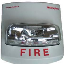
The 4906-910x Multi-Candela strobes are high output xenon strobes capable of signalling evacuation using the ISO 8201 "T3" temporal pattern, as required by AS1670.4-2004 and AS 1670.1-2004. They produce white light with a link-selectable intensity of 15cd, 30cd, 75cd or 110cd. Control is by either the ISO 8201 Strobe Driver Module (PA1043) or a QE90 STRM Strobe Relay Module (PA0697).
