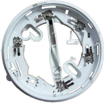
The 4B-C Continuity Base is used for most installations involving 850 Series detectors, as it allows the detector's in-built short circuit isolation function to be in-circuit when the detector is fitted and ensures continuity is maintained when the detector is removed. The 4B-C is not supported on MX4428.
