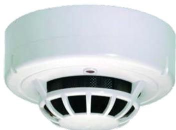
The 5351E thermal detector incorporates an Application Specific Integrated Circuit (ASIC). Combined with the latest in thermal element technology the detector provides efficient and accurate detection of fires, especially in environments such as bars or kitchens where smoke detectors are inappropriate due to the high level of airborne contamination.
