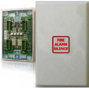
The AZM800 is a loop-powered MX Addressable module which cost-effectively integrates many of the key functions required for Type 5 fire alarm systems as defined in the NZ Building Code Compliance Documents, and in particular providing “hush”-able local alarm functions with brigade calling heat detectors and call points on the same circuit.
