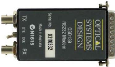
The OSD139HS Asynchronous RS232 Transceivers can interconnect one RS232 data channel over 3km of multimode fibre (OSD139HS) or over 40km of single mode fibre (OSD139HSL). These can provide complete end-to-end isolation of a full duplex asynchronous data transmission at up to 120kbps.
