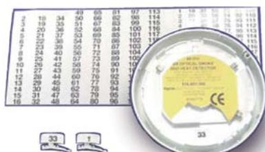
The 800 Series detectors incorporate a feature which automatically transfers the address flag to the detector base when the detector is plugged into the base. On removal of the detector the address flag is retained in the base, thus helping to ensure that detectors are not accidentally returned to the wrong detector base following service routines. Address flags are supplied in packs of 100.
