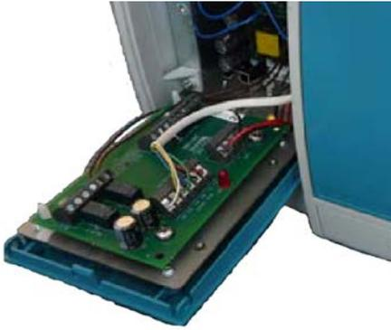
The VIO800 is an arrangement of the MIO800 Addressable Multi-I/O Module supplied ready to be fitted on to a VESDA LaserPLUS or Laser SCANNER. The MIO800's inputs and outputs are wired to the relay outputs and control inputs of the LaserPLUS or Laser SCANNER to allow compatible MX CIE to monitor and control the VESDA units.
