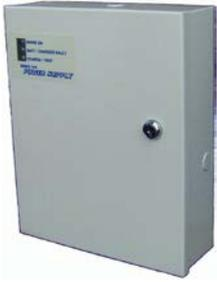
Series 1948 Power Supplies are designed specifically for use in fire alarm systems. They provide a compact, self-contained mains power supply. Their built-in facilities to monitor the charging voltage and battery capacity make them ideal for powering brigade signalling equipment, detectors, warning devices and ancillary equipment. If the charging voltage or battery capacity becomes low they activate a warning indication and output. Sealed lead-acid batteries may be purchased separately.
