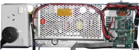
The 5A ME0476 Power Supply is a direct replacement for older 2.5A FP0874/FP0825 supplies. The ME0476 is used in MX4428 panels (or F4000 upgraded to V3.10+ software). It features a 3 pin GPO, replacing the metal mains cover & panel mount mains switch.
