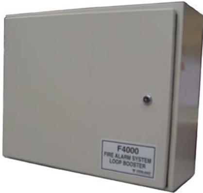
The MX4428/F4000 Loop Booster overcomes problems such as Responder loop voltage drop and excessive loop length that would otherwise necessitate a restriction in responders or the use of thicker loop cable.
