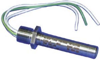
Constructed from stainless steel, the T54B is an extremely rugged heat detector that can be used to detect fires in the harshest of environments. The T54B can be used in environments with ambient temperatures up to 280°C and, being hermetically sealed, is impervious to most contaminants.
