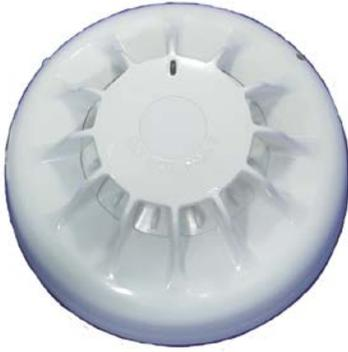
The 814H is a flexible cost-effective addressable heat detector with most of the features of *MX VIRTUAL* detectors. The 814H returns the temperature to the *MX* fire alarm panel which allows various detection modes, including all AS 1603.1 Types and many AS 7240.5 classes, to be implemented. The 814H uses a high quality thermistor with very low thermal mass. This allows the detector to function as a heat detector as well as providing a fast and accurate temperature display.
