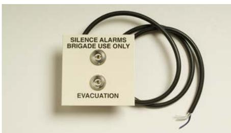
ME0433 consists of a set of (Trial) Evacuation and Silence Alarms 2-pole 2-way Bulgin keyswitches, pre-assembled and wired on a labelled White (Titania) plate. Both of these switches have their key removable in one position only to comply with NZS 4512:2003. The unit is designed to directly replace the MCP blanking plate in the standard 15U MX4428 configuration, but could also be used in other cabinet configurations, or be mounted directly to an index.
