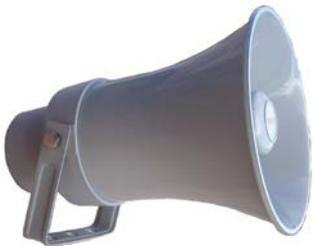
This ABS horn speaker is designed primarily for distributed paging systems where a high degree of speech articulation and program clarity is paramount. Typical applications include schools, train/bus stations, airports, car parks and plant rooms. An adjustable power tap switch is provided, as is a 22µF bipolar isolation capacitor to permit line monitoring function when employed with Warning System installations. A 4 core loop-through flying lead is provided.
