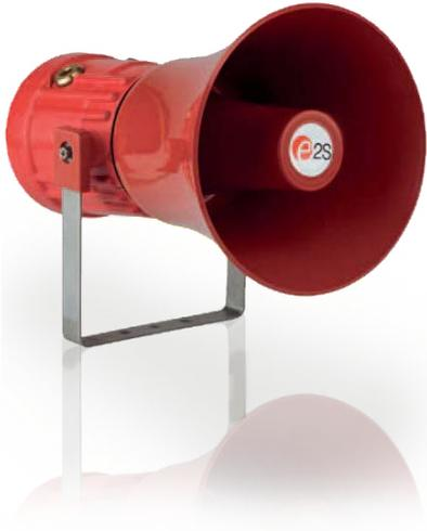
The GNEx range of flameproof PA loudspeakers is suitable for Zone 1 and Zone 2 applications. It features enclosures manufactured from GRP (glass reinforced polyester). The re-entrant flare horn is made from high impact, fire retardant ABS. The speakers have two M20 cable entries, large termination areas containing in & out terminals and an ingress protection of IP66/67. The standard mounting bracket is made from 304 stainless steel and features ratchet adjustment.
