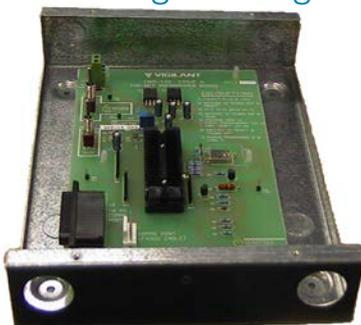
The IO-NET Programming Unit transfers the program to the IO-NET Controller PROMs. The Programming Unit is supplied complete with a cable to connect to a PC, the compiler programming software and the user manual. An external 24Vdc supply is required. IO-NET is also able to be programmed using SmartConfig Version 1.6 onwards. The IO-NET site specific configuration is stored in read-only memory. It may be re-programmed multiple times before requiring chip replacement (SF0239).
