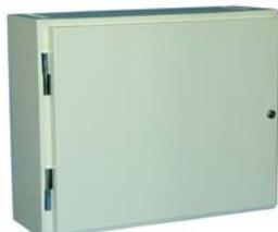
This battery box provides 8U of 19" rack capacity and has a similar finish to the range of standard Tyco 19" Rack Cabinets - 1.6mm mild steel construction, with powder coated, cream wrinkle finish. The cabinet provides IP51 protection and door is secured with 003 lock. 24 volt battery capacity is 80Ah using 2 x PS-12800 batteries (not stocked) or up to 120Ah using 6x 40Ah batteries (BA12400).
