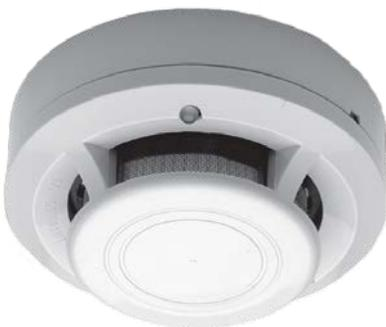
The P132A Addressable Laser Smoke Detector is a very high sensitivity smoke detector that utilises a laser photoelectric sensing chamber, providing significant improvements in signal-to-noise ratio compared with an LED light source. The detector is designed to provide open area detection for clean environments, or cubicle detection for high value equipment. The P132A Laser mounts to the B501AUS base or B200SR Sounder Base.
