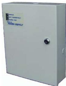
The VIGILANT 1926 DBA Power Supply is mainly intended for powering 2-wire SGD installations in DBAs but may also be used to power any fire alarm system or load where supervised 12 volt power is required. It is based on FP0765 but additionally includes a defect (battery monitor) circuit with relay contact output which is usually wired in series with the defect input of one of the SGDs it powers.
