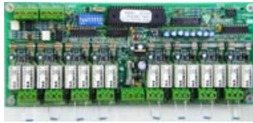
PA0697 STRM9502 Strobe/Relay Module PCB with AS 2220/ISO 8201 Selection
