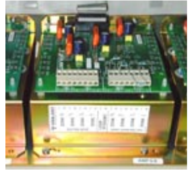
PA0795 TRAN9706-1 4x10W Transformer Module without Relays
