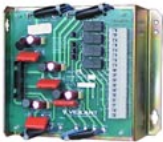
PA0796 TRAN9706-2 4x10W Transformer Module c/w Relays
