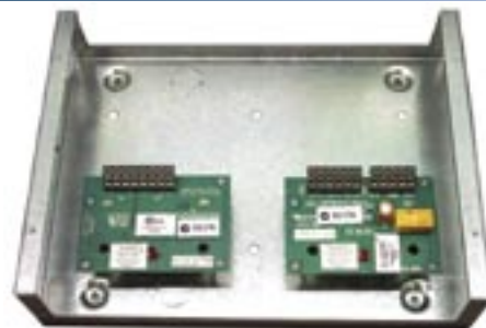
FP0529 Empty Responder Box showing MX modules fitted
