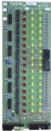
Display Extender PCB 248x98mm
