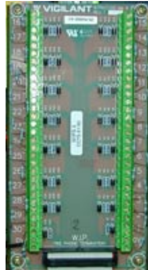
PA0916 WTRM2000 WIP Termination PCB
