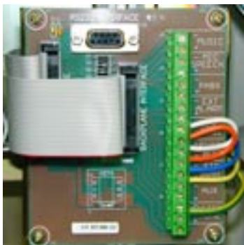
PA0657 SE9004 Signal Interface PCB
