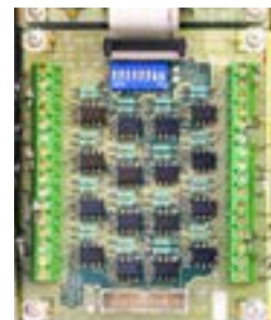
PA0652 FIPE9004 FIP/BGA Extender Module
