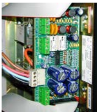
PA0691 HTRN9308-1 2x50W Transformer Module
