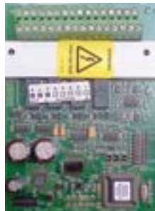
4100-3204 4 Aux Relay + Feedback PDI Card
