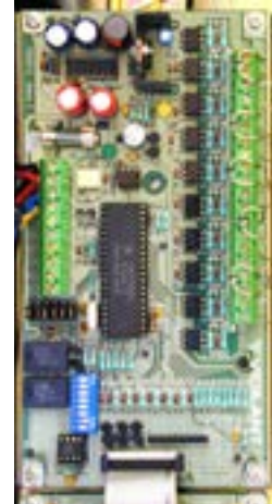
PA0651 FIB8910 FIP/BGA Master Module DD0084 FIP EOL Zener Diode
