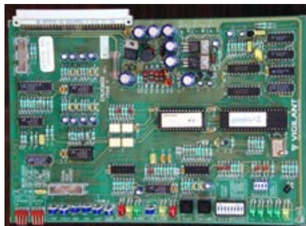
PA0758/759 EMUX9601 Multiplexer 16/60s Speech with AS 2220 and ISO 8201 Selection
