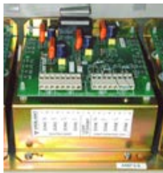
PA0795 TRAN9706-1 4x10W Transformer Module without Relays
