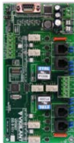
PA0644 VIF0907 VolP Interface incl. 1x LM0448, 2x LM0552, DIN rail mntg h'ware
