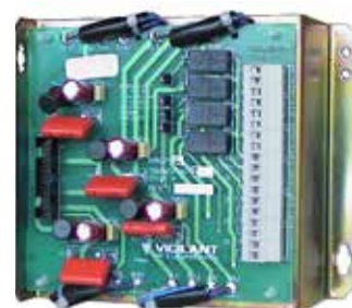
PA0796 TRAN9706-2 4x10W Transformer Module c/w Relays
