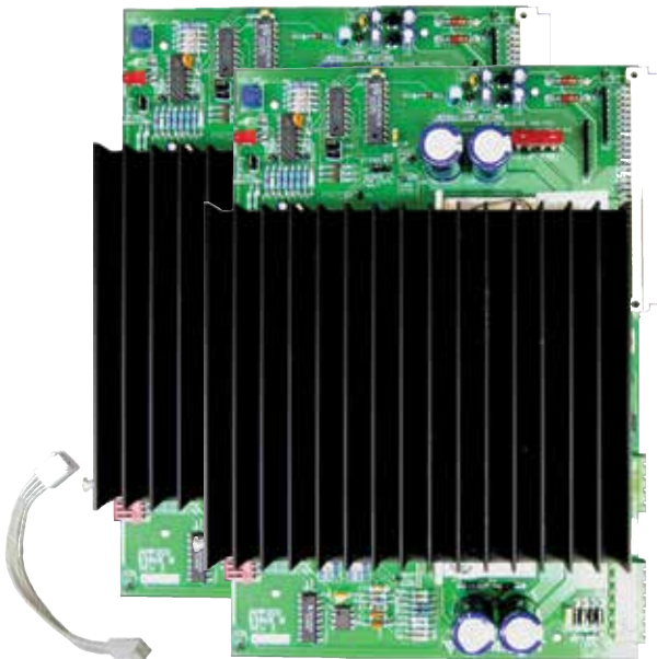
KT0519 200W Amplifier Module Kit The 200W amplifier comprises two PA0647 AMP200 PCB modules and one LM0141 FRC loom.
