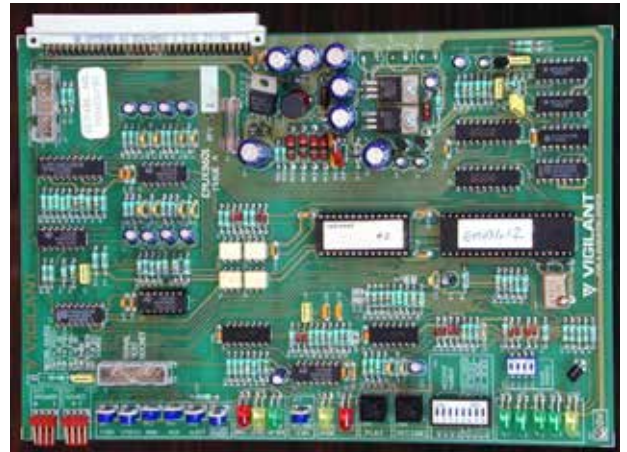
PA0758/759 EMUX9601 Multiplexer 16/60s Speech with AS 2220 and ISO 8201 Selection
