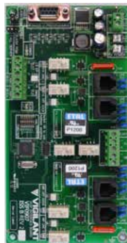
PA0644 VIF0907 VoIP Interface incl. 1x LM0448, 2x LM0552, DIN rail mntg h'ware
