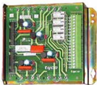
PA0792 TRAN9705-2 4x25W Transformer Module c/w Relays
