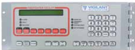
The Network Display Unit (NDU) is a fire alarm repeater panel compatible with the Panel-Link Network and the associated range of networked fire alarm systems (eg. MX4428, F3200). It provides alphanumeric display of alarms on a 2 line by 40 character LCD and keypad. The NDU is able to display alarms and status, and control all fire alarm panels connected to the network.
