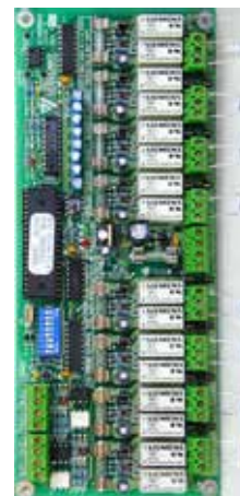
PA0697 STRM9502 Strobe/Relay Module (WEB) with AS 2220/ISO 8201 Selection
