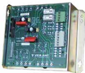
PA0794 TRAN9705-4 2x25W Transformer Module c/w Relays
