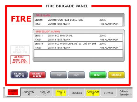
The first alarm to occur is displayed in the FIRST ALARM section of the Alarms tab.
